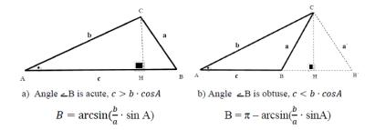
Figure 1: Examples of SAS theorem when a) the angle B is acute and b) when it is obtuse.
