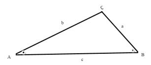
Figure 2: ASA theorem: given are the angle A, the angle B, and the side c.
